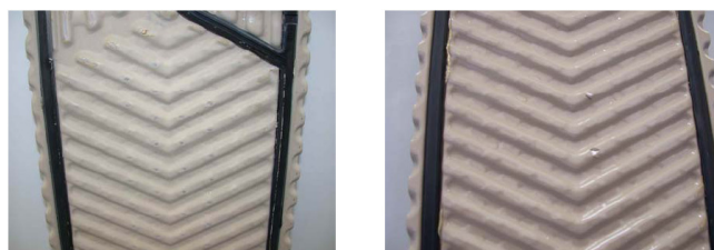
Coated heat exchanger plates with nano-technology
