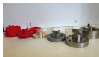
Figure 5. Left to right (1 to 5 front row) From conceptual prototyping in ABS departmental printer to 3D printing of functional moulds in PPSF (3) and Aluminium (4) before final production of a final stainless steel die
