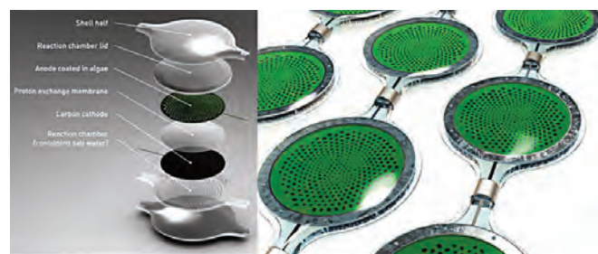
Figure 4. A BPV solar panel array (right) could be a useful household power supplement. Based on designs from the Cambridge Institute for Manufacturing (left), prototypes are currently being tested (see Figure 2)
