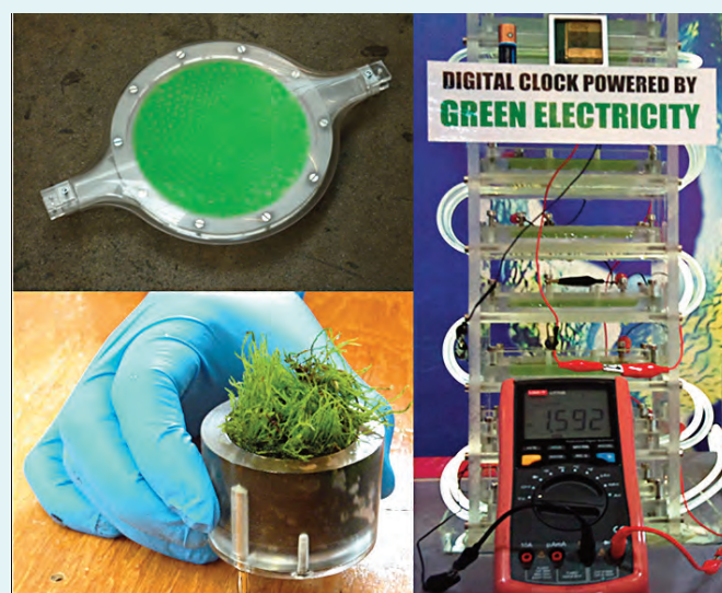
Figure 2. Current BPV prototypes produced at the University of Cambridge. Algae (top left and right) and moss (bottom left) designs can presently produce enough energy to power small electronic devices.
