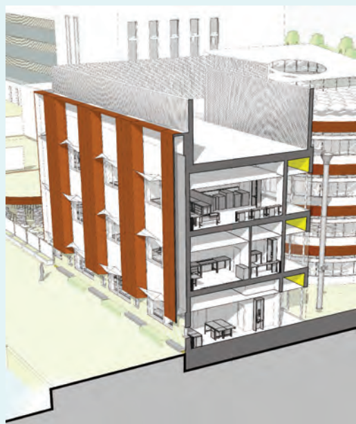
Cutaway perspective of the work in progress Revit model showing the laboratory fit-out model combined with the structural and architectural model
