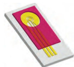
Figure 1. Schematic illustration of the chip highlighting the arrangement of three Au electrodes system
