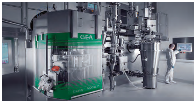
Picture from GEA pharma section, demonstrating a production on demand (POD) mini-factory. www.tinyurl.com/o6by69c
