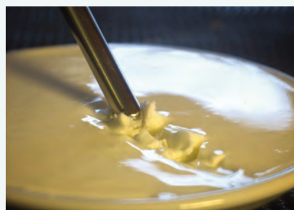
A shear thickening suspension reversibly solidifies as a large stress is applied
