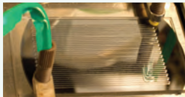
A Si-glass microfluidic reactor frequently used in the group to study reactions under flow conditions.
