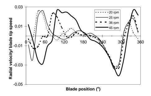
Fig. 8 : Ratio of the radial velocity of the tracer to the blade tip speed vs. blade position, influence of the agitator speed; level of fill :60%
