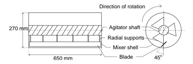
Fig. 1 : Sketch of the mixer : side and cross-sectional views
